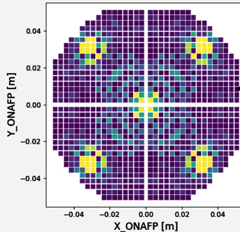
**PSF** : Response of the instrument on the focal plane for one direction on the sky, at one wavelength.
