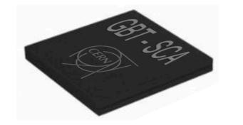
The GBT-SCA ASIC (Giga-Bit Transceiver - Slow Control Adapter) is the part of the GBT chipset which purpose is to distribute control and monitoring signals to the front-end electronics embedded in the detectors.
