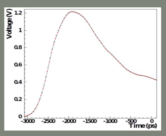
• Timing with CFD at 20% of peak amplitude
