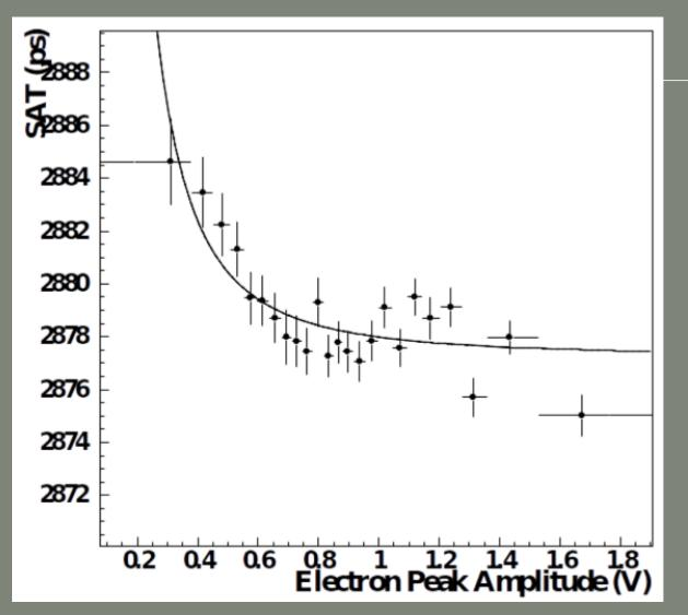
• In principle, CFD method DOES NOT suffer from time walk effect • However, we observe a dependence of the SAT on the signal amplitude
