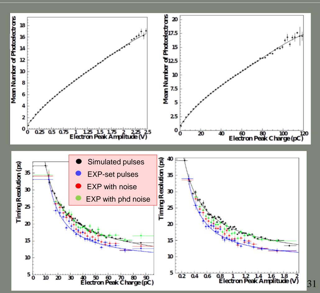
• Timing with Timing threshold at 100mV and multi-Charge over threshold corrections
