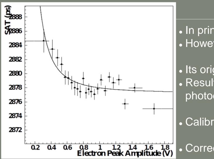
• In principle, CFD method DOES NOT suffer from time walk effect • However, we observe a dependence of the SAT on the signal amplitude
