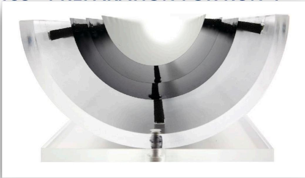
bending silicon chips thinned down to  $30\text{-}50\mu\text{m}$
