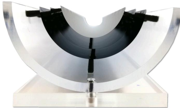
wafer-scale MAPS sensors curled around beam pipe
