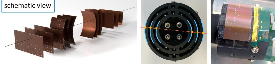
Full-size prototype of half-layers (unprocessed silicon)
