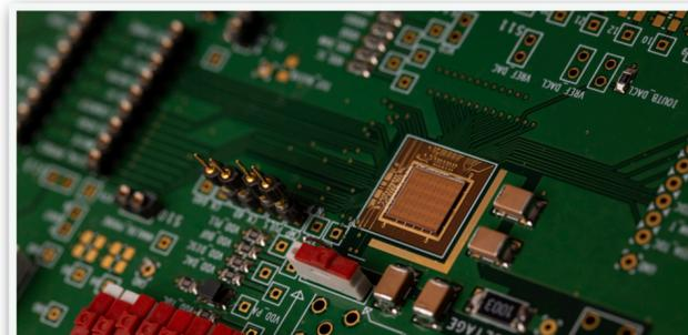
Altiroc HGTD readout chip prototype
