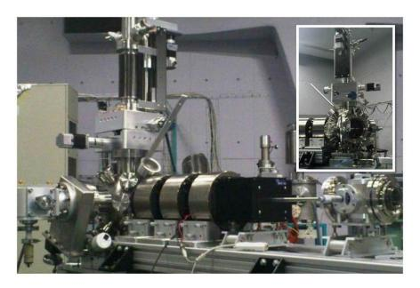
Nuclear micro-probe (beam spot on sample Ø≈1 µm) dedicated to the analysis of cultural heritage objects, biological samples, aerosol filters etc.
