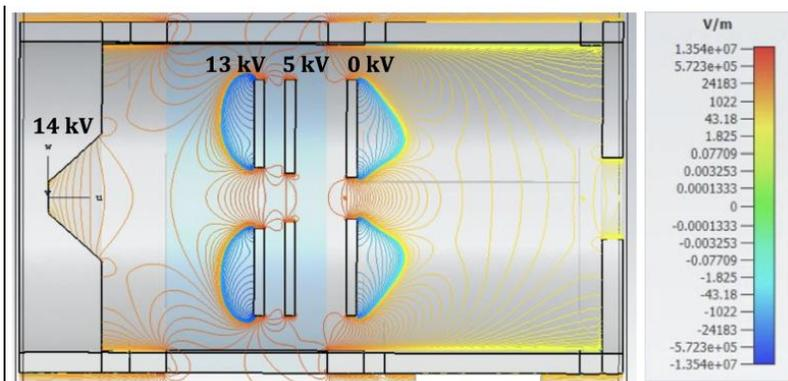
Figure 6.23: Equipotential lines and electric field values for 3D model of the extraction system geometry.
