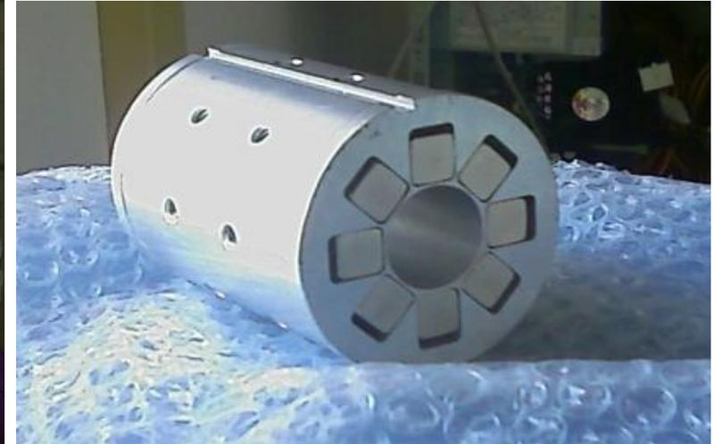
PMQ for tank2 , 60 mm in diameter and 80 mm in length
